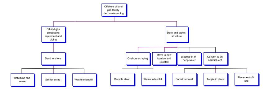
Figure C.10. Offshore Oil and Gas Facility Decommissioning Tree.
